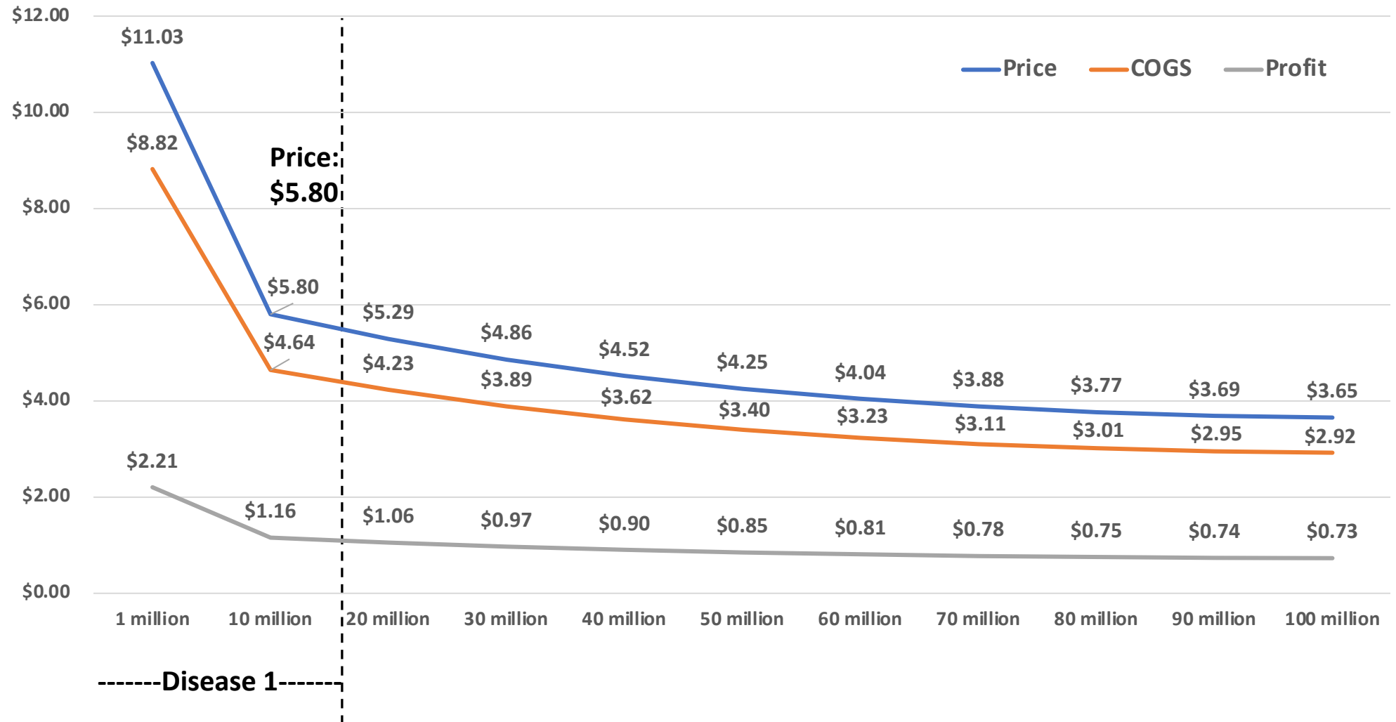
Model of volume-based variation in evidence-based price, COGS, and profit for molecular tests, based on estimated COGS of GeneXpert tests
